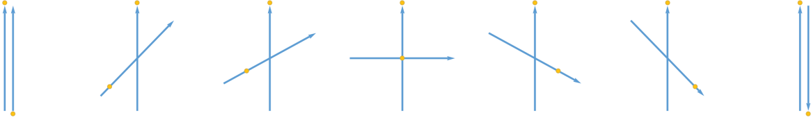
Figure 6. Average View for the Spin Singlet State. Reading from left to right, as Bob rotates his SG magnets relative to Alice’s SG magnets for her +1 outcome, the average value of his outcome varies from -1 (totally down, arrow bottom) to 0 to +1 (totally up, arrow tip). This obtains per conservation of spin angular momentum on average in accord with no preferred reference frame. Bob can say exactly the same about Alice’s outcomes as she rotates her SG magnets relative to his SG magnets for his +1 outcome. That is, their outcomes can only satisfy conservation of spin angular momentum on average in different reference frames, because they only measure \pm 1 , never a fractional result. Thus, just as with the light postulate of special relativity, we see that no preferred reference frame leads to a counterintuitive result. Here it requires quantum outcomes \pm 1 (\frac{\hbar}{2}) for all measurements and that leads to the “mystery” of “average-only” conservation. Note: Here you can see the physical reason that \theta = 2\Theta for spin- \frac{1}{2} particles found in Methods, i.e., spin is a bi-directional property in the plane of symmetry for spin- \frac{1}{2} particles.
