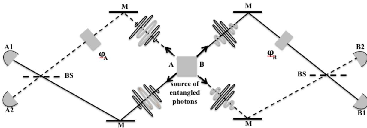
**Figure 4.** The RTO experiments. In each trial, each of two entangled photons travels two phase-shifted paths (one solid, the other dashed) to beam splitters and coincidence detectors. Think of one biphoton spreading from the source along both the solid and the dashed paths.
