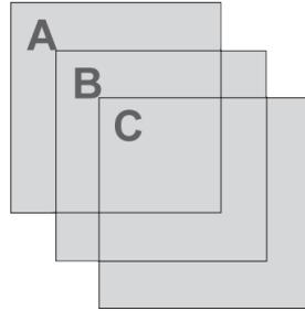
When polarizers A and B are superimposed we see that the same amount of light comes through two polarizers, as long as the polarizing direction is the same. The first polarizer A prepares the photon in a given state of polarization. The second is then certain to find it in the same state. Let's say the direction of light polarization is vertical when the letters are upright.
